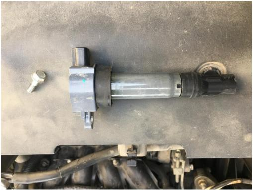
3. Select the appropriate adapter (some cars do not require an adapter to directly use an extended aluminum tube), and screw the extended aluminum tube into the ignition coil.
